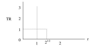
Note that for all values of damping ( $\zeta$ ), the transmissibility ratio equals one (TR=1) at both r = 0 and at  $r = \sqrt{2}$ . The maximum transmitted force will always occur at  $\omega_f < \omega_n$  regardless of the system characteristics (m, k, c). The frequency ratio for maximizing the transmitted force, is  $r_{TRmax}$  and is given by:
