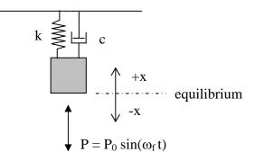
In addition to the inertial force, there are three forces acting on the mass: the spring force (proportional to displacement), the force from the dashpot (proportional to velocity) and the external force, P. All of these forces are a function of time. The free body diagram (FBD) is:
