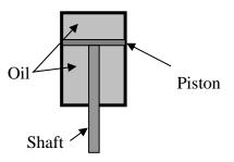
Holes in piston allow oil to flow from one side to the other (viscous forces are produced). Various relationships between velocity and force can be created by varying design:
