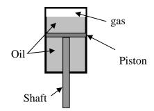
The system we will study consists of a mass, spring, and dashpot (shock absorber). The dashpot is viscous (force is proportional to velocity).
