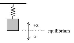
If a system is displaced from equilibrium it will move to seek out equilibrium. If there is no damping, the system will continually convert energy back and forth between kinetic energy of the moving mass and elastic energy of the spring.
