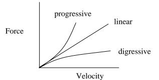
Progressive and digressive shock absorbers can be created by using shims (flaps) to partially cover the passage holes in the piston giving a non-linear response. This can also be used to create a different response depending on the direction of travel (up verses down for example). We will only consider linear response (force is directly proportional to velocity).
