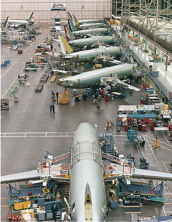
737 - OLD ASSEMBLY STATIONS
