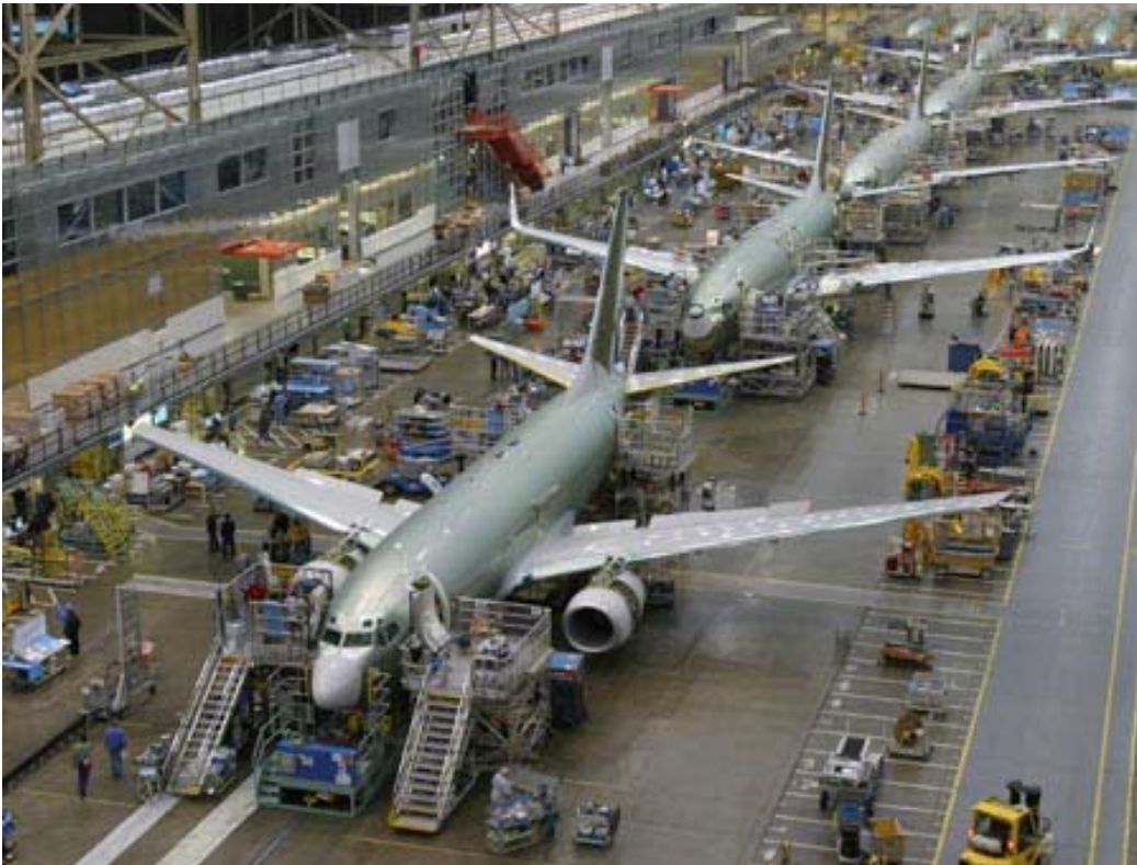
MOVING ASSEMBLY LINE, 737
