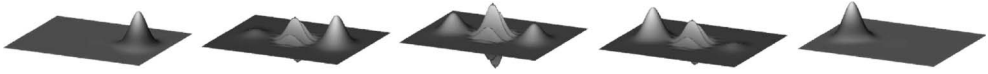
Fig. 2. Time evolution of the Wigner function corresponding to a superposition |\Psi(t)\rangle \propto |L\rangle \cos(\Delta Et/2) + i|R\rangle \sin(\Delta Et/2) of the two localized opposite-current states |L\rangle and |R\rangle in a SQUID. The state coherently oscillates between the two wells, leading to coherent quantum tunneling. This manifests itself in a macroscopic current oscillating between clockwise and counterclockwise directions. Figure reprinted with permission from [39]. Copyright 2004 by the American Physical Society.
