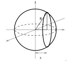
(*iv*) The area of the cross section at x is  $\pi (R^2 - x^2)$ .
