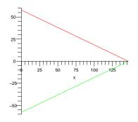
Notice that the side of the pyramid follows the line  $57.85 - \frac{57.85}{146.59}x$ , so at the point x, **half** of the side of the square is  $57.85 - \frac{57.85}{146.59}x$ . Hence  $A(x) = (115.7 - \frac{115.7}{146.59}x)^2 = \frac{(115.7)^2}{(146.59)^2}(146.59 - x)^2$ , so we get  $V = \int_0^{146.59} \frac{(115.7)^2}{(146.59)^2}(146.59 - x)^2 dx$   $= -\frac{(115.7)^2}{3 * (146.59)^2}(146.59 - x)^3 \Big|_0^{146.59} = 654109.$
