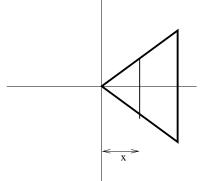
From a simple sketch (see illustration), we see that at the point x, the length of half of one of the sides is  $x \tan(\pi/6) = \frac{\sqrt{3}x}{3}$ , so the length of one of the sides of the square at x is  $2\sqrt{3}x/3$ . This means the area of each cross-section will be  $A(x) = \frac{4}{3}x^2$ , so we get
